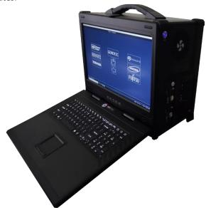
GENESIS two channel controller with embedded com port to connect up to two source drive at the same time.
