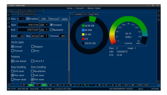
Friendly user graphic interface makes easy to create image file or physical copy to load into extraction software. With genesis is possible to stop a task and resume when needed without starting each time from zero, a map of skipped sectors will be created for report creation
